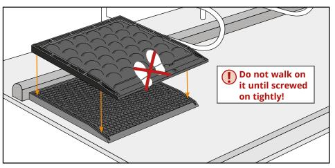
The stud links of the upper mat engage in the edge of the lower mat
