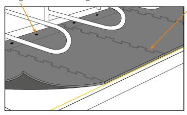
Puzzle interlock system does not depend on the divider arrangement
