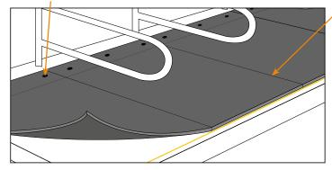
Puzzle interlock system or joint roughly underneath the divider (max. +/- 8 cm)
