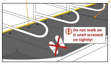
Puzzle interlock system or joint roughly underneath the divider (max. +/- 8 cm)
