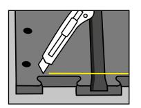
Any excess puzzle pieces can be cut off at the start and end of an area.
