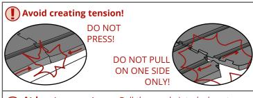
At low temperatures: Pull the puzzle interlock system apart to create a visible gap.
