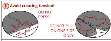
At low temperatures: Pull the puzzle interlock system apart to create a visible gap.
