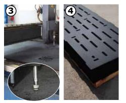
based on the CAD created drawing, the slits are cut exactly into the mats with innovative water jet technology
