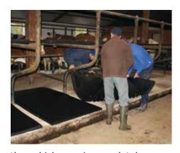
the cubicle row is completely covered with the mats
