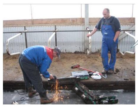
**tip:** turn scraper over, check for sharp edges and if necessary deburr them with an angle grinder
